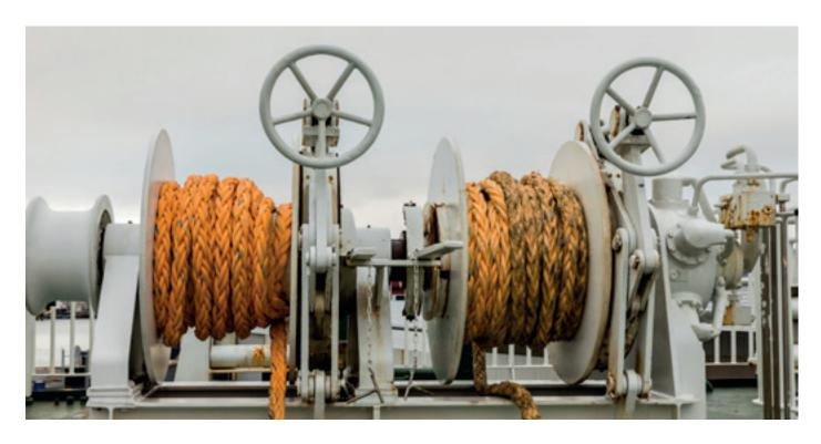
Any rope that has been in use for any period of time will show signs of wear and tear, some characteristics of use will not reduce strength while others will. Ropes should be inspected on a regular basis for wear and tear and any faults / repair / retirement required.
